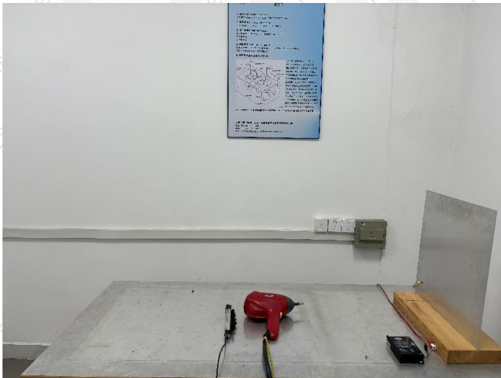
Photograph 2 :Setup for Electrostatic Discharge
